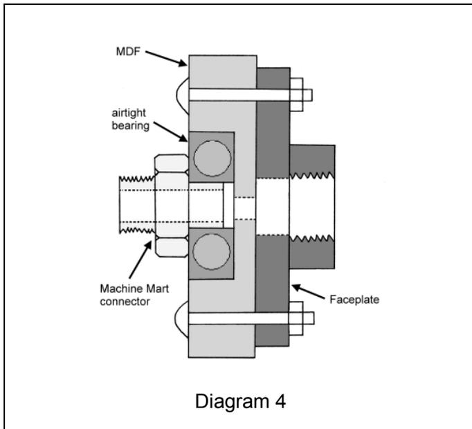
A few drops of superglue were smeared round the edge of the hole and the bearing was pushed into place. Another hole was drilled through the centre of the MDF in line with the centre of the bearing.
