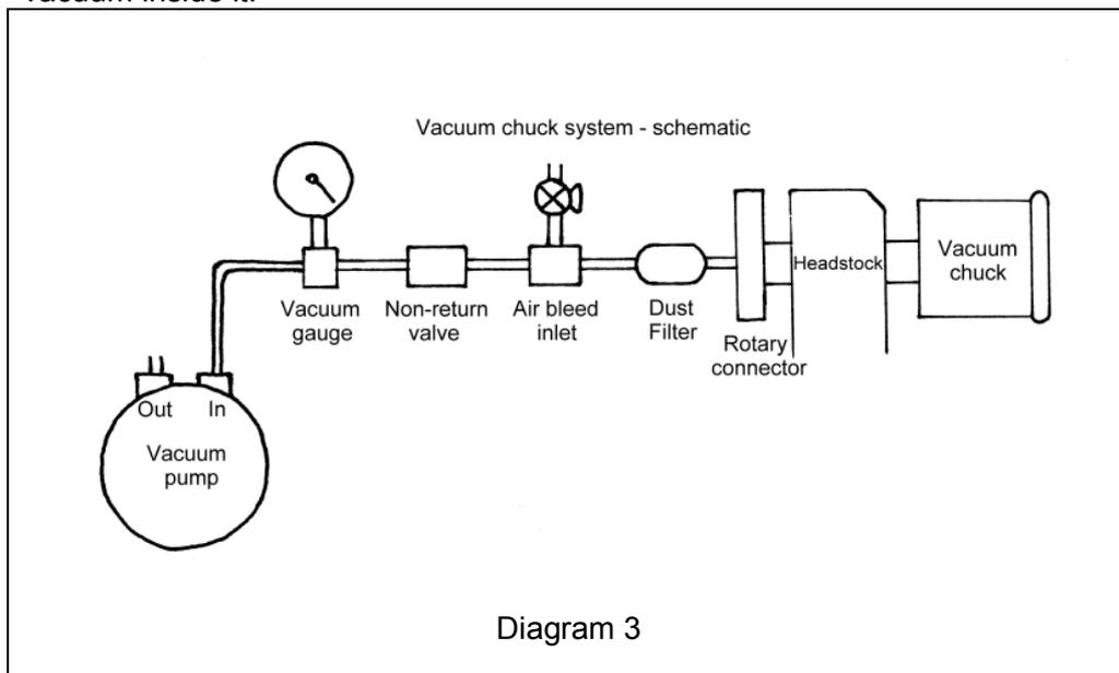
**Diagram 3** shows the layout in principle but when I actually put it together I 'folded' it to make it smaller and neater (**Photo 4**).
